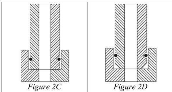
To minimize the distance alloy must travel after melting, particularly where a large area is to be joined, it is sometimes advantageous to provide a groove where the alloy may be placed during assembly. Depending on its location, this groove can
