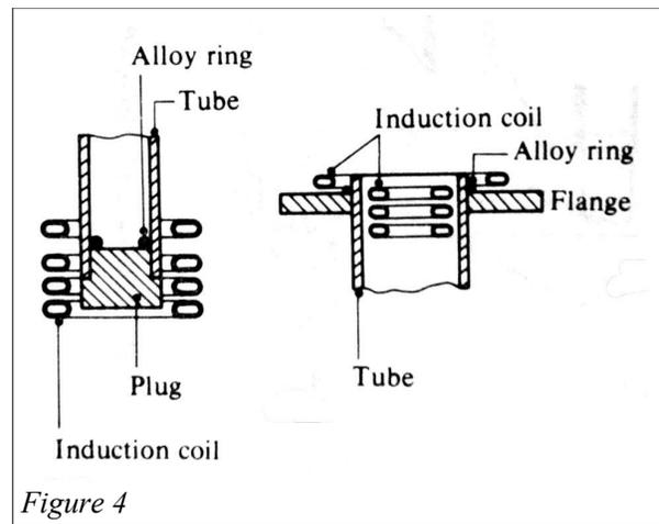
Typically, in a tool-brazing system where the steel has a lower resistivity than the tungsten carbide insert, as well as a greater mass, the coil is positioned lower on the tool to deliver more heat to the steel shank. See Figure 4.
