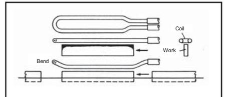
**Fig. 9: Typical channel coil used to heat the edges of discrete lengths of rectangular bar stock; end of coil is decoupled by bending to prevent overheating of ends (from F. W. Curtis, *High Frequency Induction Heating*, McGraw-Hill, New York, 1950)**
