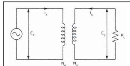
$E_p$  = primary voltage (V);  $I_p$  = primary current (A);  $N_p$  = number of primary turns;  $I_s$  = secondary current (A);  $N_s$  = number of secondary turns;  $E_s$  = secondary voltage (V);  $R_l$  = load resistance ( $\Omega$ )
