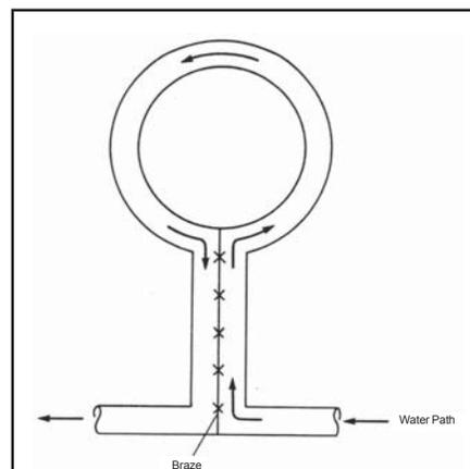
Fig. 19: Typical construction of a water-cooled flux robber.
