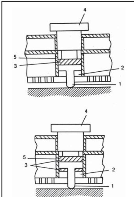
**Fig. 5: Design of metal and ceramic pins for fixing the position of a split inductor on a crankshaft journal (from M.G. Lozinski, *Industrial Applications of Induction Heating*, Pergamon Press, London, 1969)**
