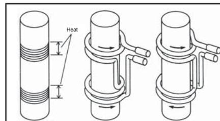
Fig. 17: Control of heating patterns in two different regions of a workpiece by winding the turns in opposite directions (from F. W. Curtis, *High Frequency Induction Heating*, McGraw-Hill, New York, 1950)
