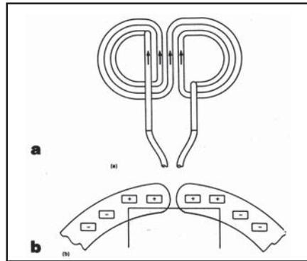
**Fig. 6: Schematic illustration of a butterfly coil: (a) coil construction (arrows indicate reinforcing type of current flow in coil); and (b) coupling between the turns of the coil and the end of a bar to produce a uniform heating pattern**
