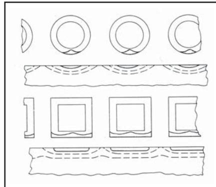
Fig. 1: Comparative heating patterns produced by using round vs. square tubing for a solenoid induction coil (from M. G. Lozinsky, *Industrial Applications of Induction Heating*, Pergamon Press, London, 1969)
