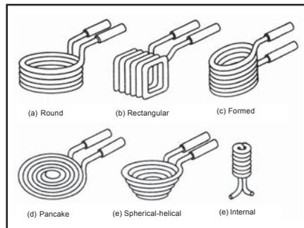
Fig. 5: Multiturn coils designed for heating parts of various shapes: (a) round; (b) rectangular; (c) formed; (d) pancake; (e) spiral-helical; (f) internal (from F. W. Curtis, *High Frequency Induction Heating*, McGraw-Hill, New York, 1950)
