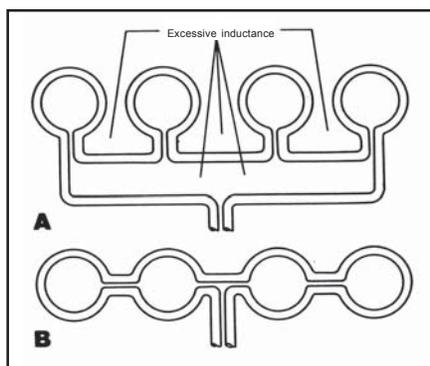
Fig. 5: Lead construction for multiplace inductors; lead design in (b) is preferable because of lower heat inductance (from F.W. Curtis, *High Frequency Induction Heating*, McGraw-Hill, New York, 1950)
