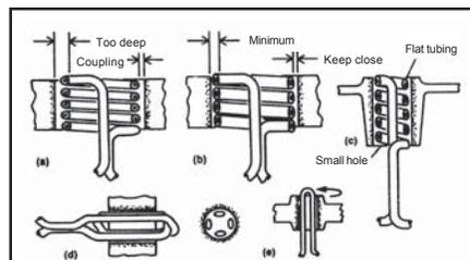
Fig. 7: Induction coils designed for internal (bore) heating (from F. W. Curtis, *High Frequency Induction Heating*, McGraw-Hill, New York, 1950)
