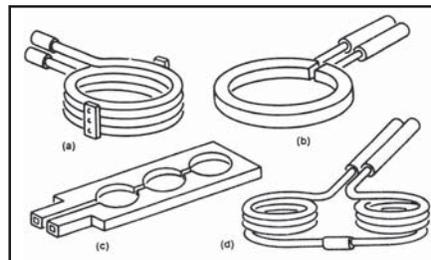
Fig. 4: Typical configurations for induction coils: (a) multiturn, single place; (b) single-turn, single place; (c) single-turn, multiplace (from F. W. Curtis, *High Frequency Induction Heating*, McGraw-Hill, New York, 1950)
