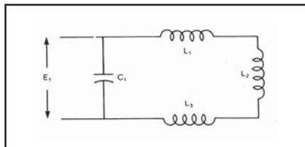
Fig. 3: Schematic circuit diagram indicating the inductance of the coil leads and induction coil itself:  $L_1$ ,  $L_3$ -lead inductances;  $L_2$ -induction-coil inductance;  $C_1$ -tank capacitance;  $E_1$ -tank voltage
