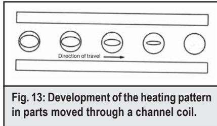
Fig. 13: Development of the heating pattern in parts moved through a channel coil.
