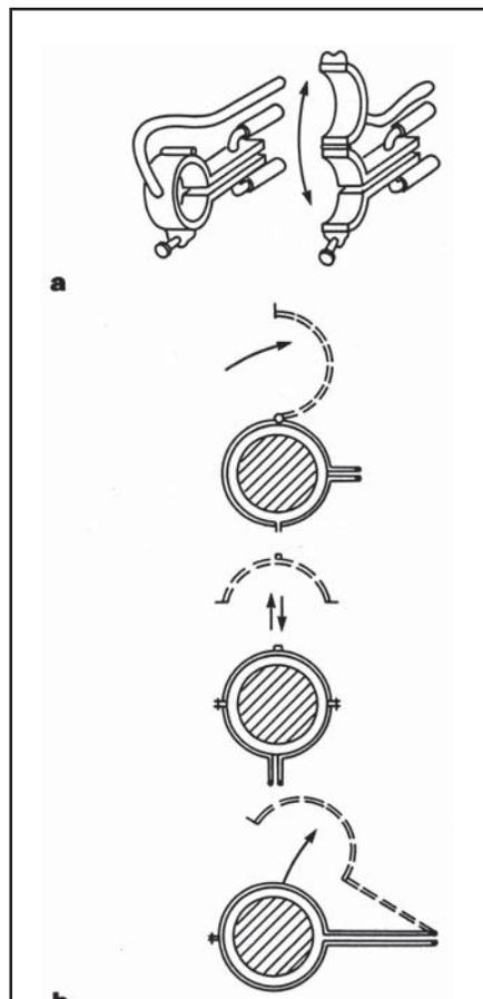
**Fig. 4:** Diagram (a) and schematic illustration (b) of a split inductor used for heating crankshaft journals (from M.G. Lozinski, *Industrial Applications of Induction Heating*, Pergamon Press, London, 1969)
