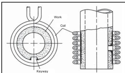
Fig. 14: Localized overheating of sharp corners, keyways, and holes most prevalent in high frequency induction heating (from F. W. Curtis, *High Frequency Induction Heating*, McGraw-Hill, New York, 1950)
