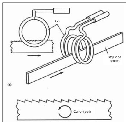
**Fig. 8: Illustration (a) of one type of transverse coil for heating a thin section; sketch in (b) indicates the current path in the workpiece (from F. W. Curtis, *High Frequency Induction Heating*, McGraw-Hill, New York, 1950)**
