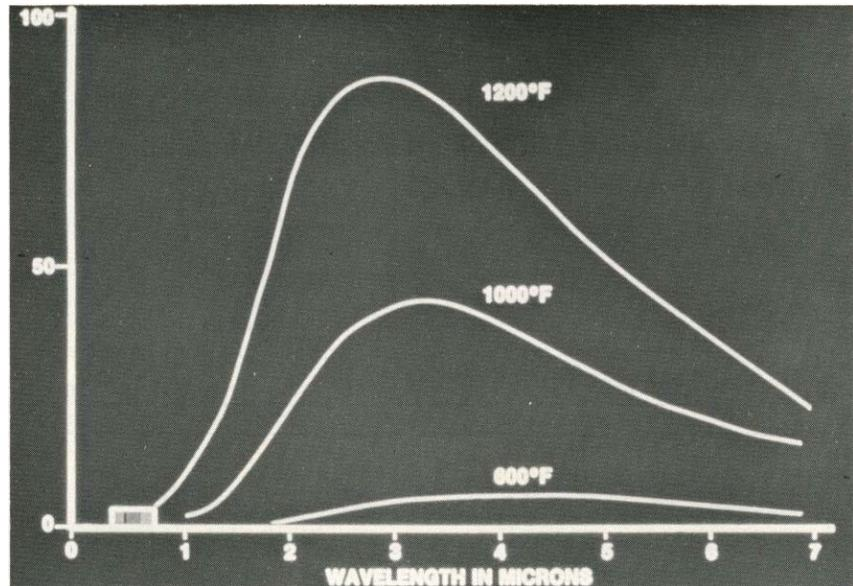
Shown here is a series of emissivity curves. As they intersect a single wavelength, a change in temperature reflects a change in signal.
