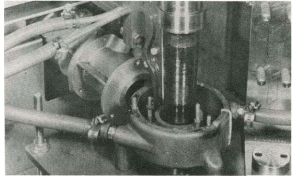
The temperature of a boiling surface is observed by the pyrometer which looks through the quench ring and coil turns
